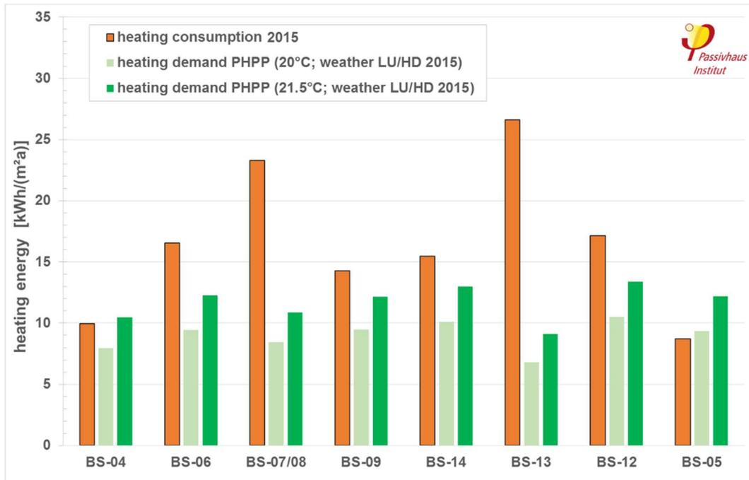
**Fig. 18: Comparison of the consumption data for heating energy (orange) with the PHPP demand values for the weather data set HD/LU 2015 and different indoor temperatures for the now eight investigated building sites in the Bahnstadt district. All buildings were fully inhabited in the year 2015.**
