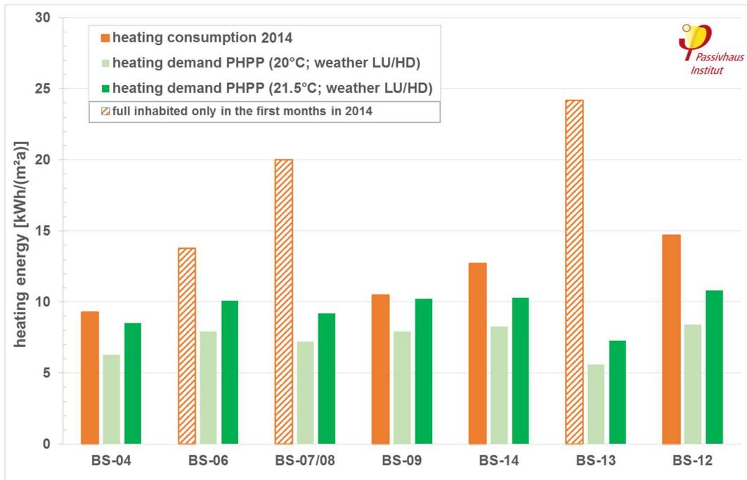
**Fig. 17: Comparison of the consumption data for heating energy (orange) with the PHPP demand values for the weather data set HD/LU 2014 and different indoor temperatures for the seven investigated building sites in the Bahnstadt district (measurement error in the range of  $\pm 4$  kWh/(m²a)).**
