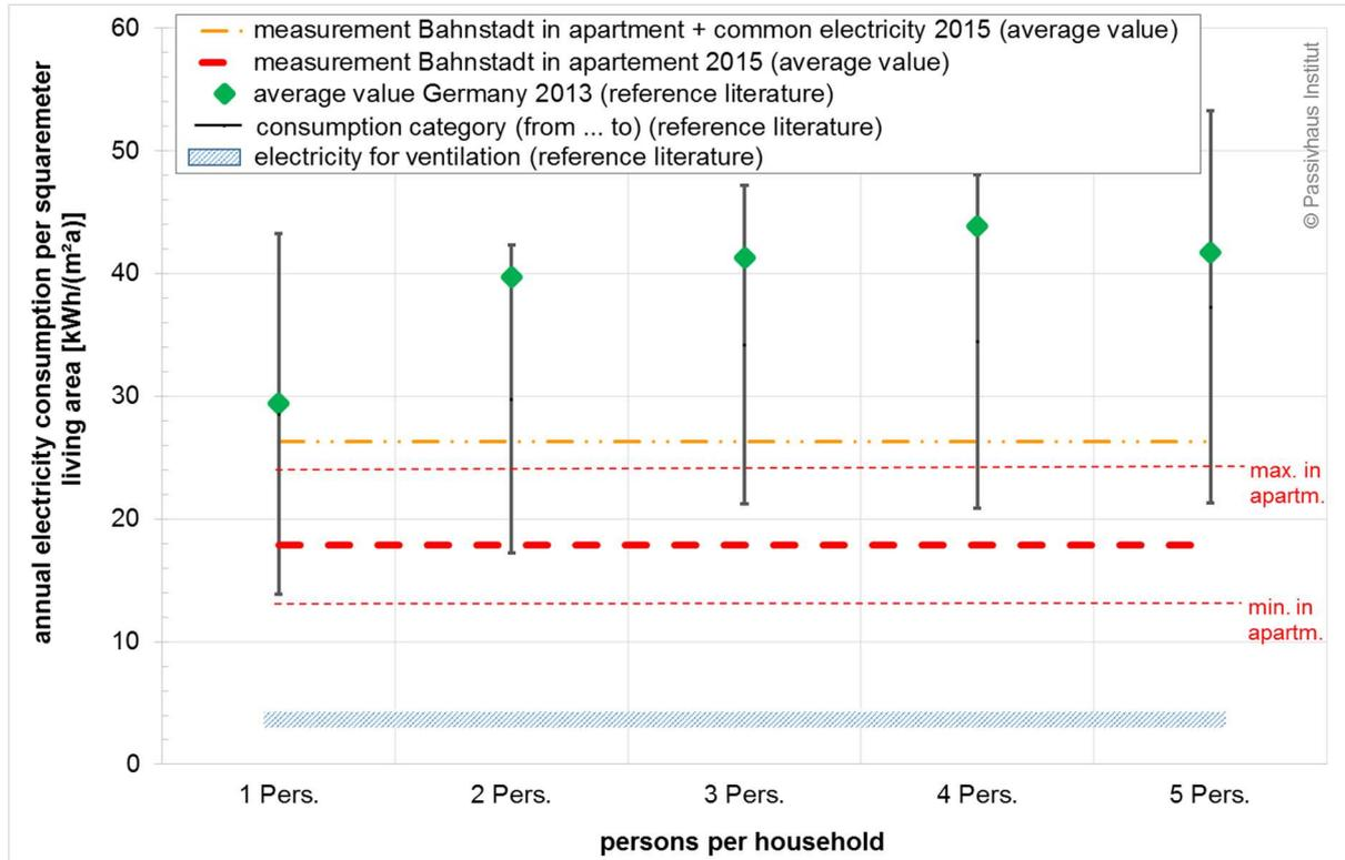
**Fig. 24: Comparison of the measured electricity consumptions in the Bahnstadt district (2015) with average values taken from reference literature (see text for explanation). The electricity for underground car parks has not been plotted here.**
