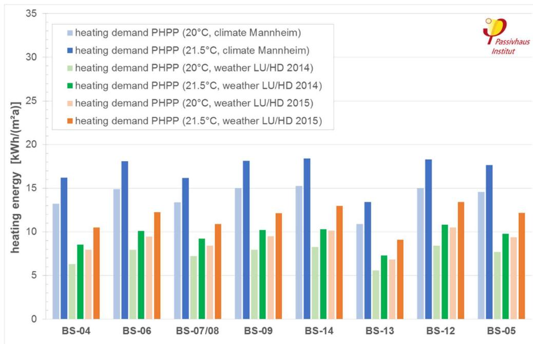
**Fig. 16: Comparison of the demand values for heating energy in the PHPP calculations for the different climate/weather data sets and indoor temperatures in the studied building sites of the Bahnstadt district in both studied periods.**
