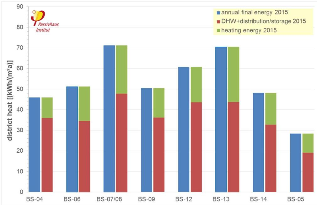
**Fig. 7:** Depiction of the annual consumption values for district heat for the year 2015 (see text for Fig. 6 for explanation). Evaluation of an additional building site was possible for the year 2015.
