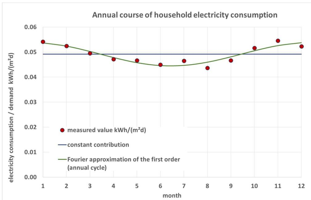
**Fig. 26:** Harmonic approximation of the annual period for the measured specific household electricity consumptions. The consumption shows a cosinusoidal annual cycle in good approximation (phase shift 14 days before the end of the year) with an amplitude which amounts to 9.5% of the average consumption.
