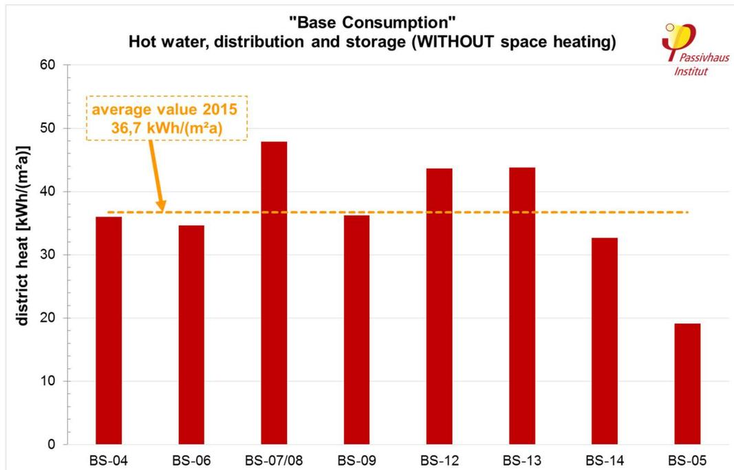
**Fig. 10: Annual district heat consumption for the so-called "base consumption" (hot water, distribution and storage without space heating) of the residential-use buildings (including the student hostels) separately according to building sites for the year 2015 (taken from Fig. 7).**
