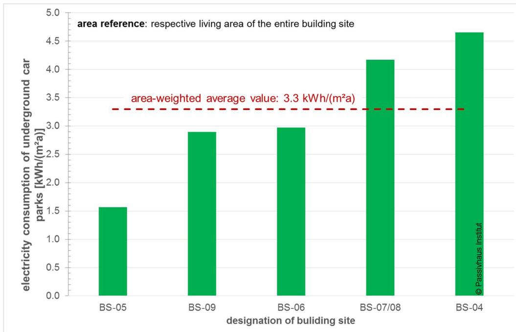
**Fig. 23: Specific electricity consumption for operation of the communal underground car parks for each building site. The living area (treated floor area) of the entire building site (total buildings) is used as the area reference. In this way, these values can be directly compared with the other consumption data.**
