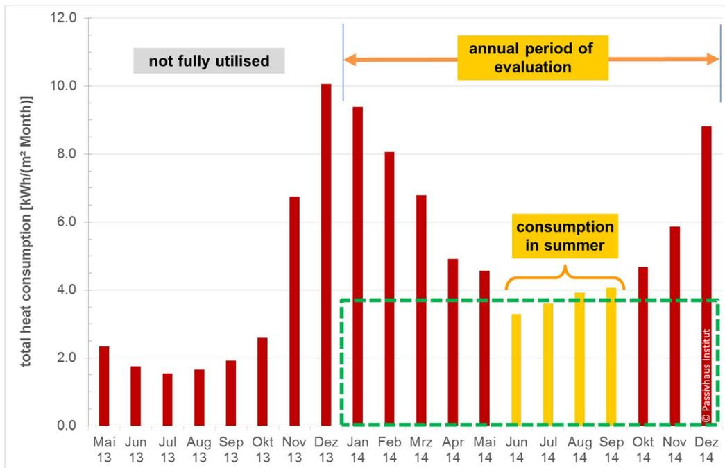
**Fig. 4: Monthly consumption values for district heat in an example building site in the Bahnstadt district in Heidelberg. The method for determining the heating energy consumption is explained in the text.**
