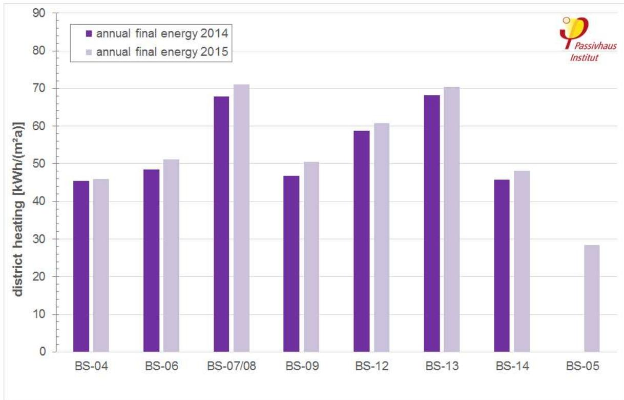
**Fig. 5: Annual measured consumption values for "total district heating" for residential use (including student hostels) according to building sites for the calendar years 2014 and 2015.**
