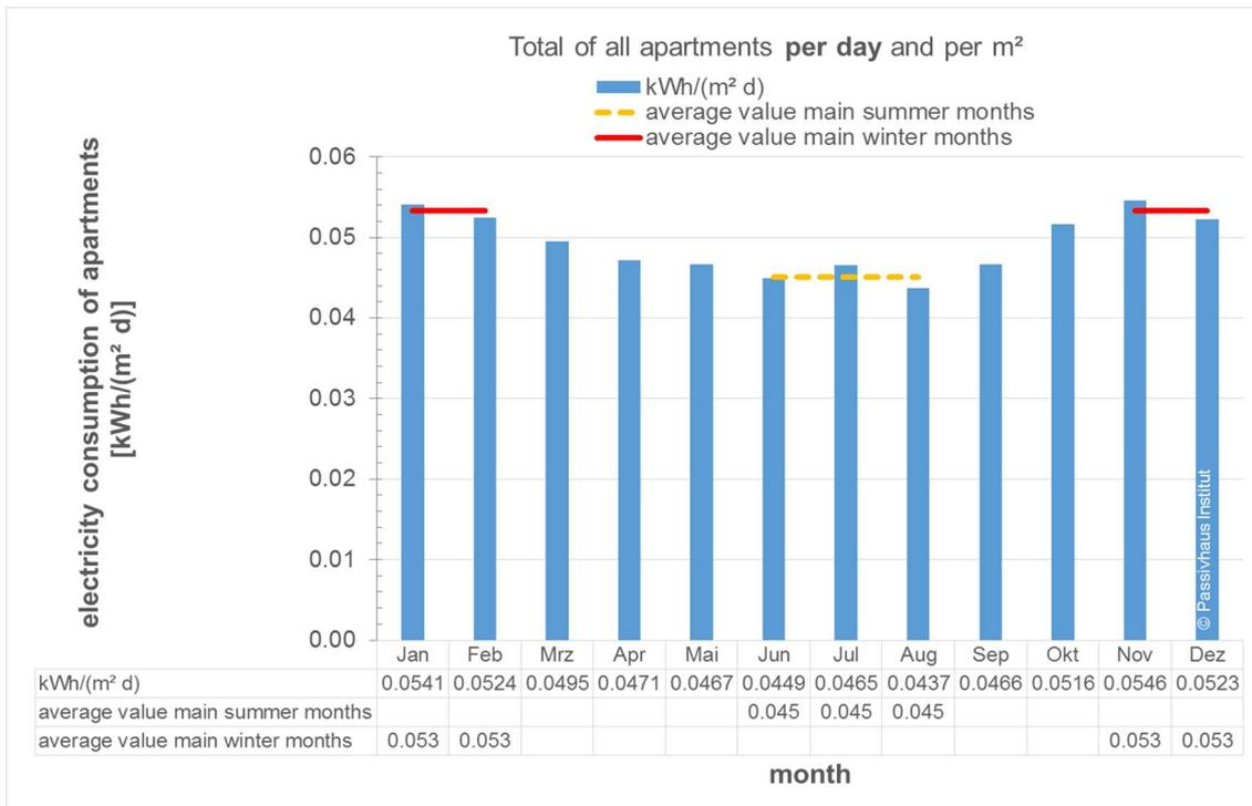
**Fig. 25: Average monthly electricity consumption values for the household electricity for all studied buildings translated to specific daily average consumption values. The average values of the three main summer months and the four main winter months have been indicated in the graph.**
