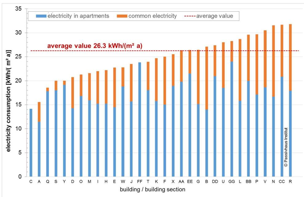
**Fig. 22:** Specific electricity consumption of the 33 buildings in Fig. 21 in the Bahnstadt district of Heidelberg in the year 2015 with the common electricity consumptions added (without the electricity consumption of the underground car parks). The area-weighted average value is 26.3 kWh/(m²a).
