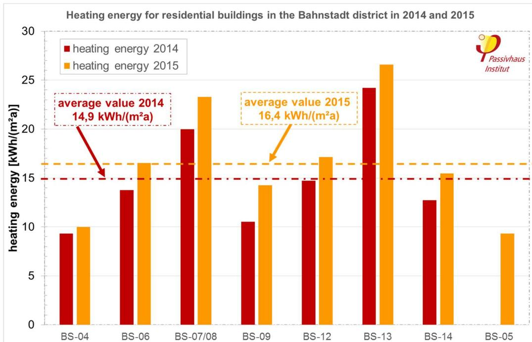
**Fig. 11: Annual heat consumption values in the Bahnstadt district for residential-use buildings (including student hostels) separately according to building sites (taken from Fig. 6 and Fig. 7) for both studied years (error analysis:  $\pm 4$  kWh/(m<sup>2</sup>a)).**
