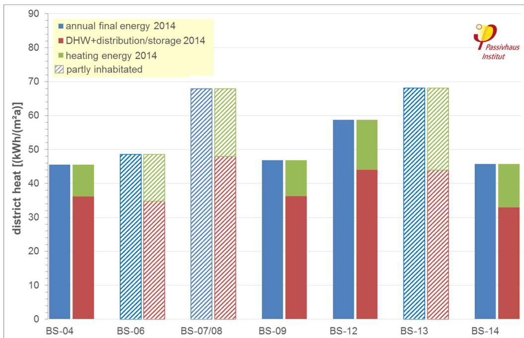
**Fig. 6: Annual consumption values for district heat in 2014 for residential use buildings (including student hostels) according to building sites. The total consumption (blue) is divided into space heating (green) and the remaining consumption (red) according to the method described in Section 2.2. The building sites indicated with shading were only fully inhabited after one to three months in the year 2014 ("partly inhabited").**
