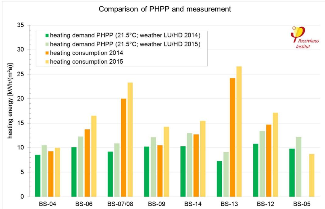
**Fig. 19: Comparison of the PHPP demand values for heating energy at a temperature of 21.5 °C with the measured consumption data for both investigated years. The increases from 2014 to 2015 can be explained by the change in the weather conditions.**
