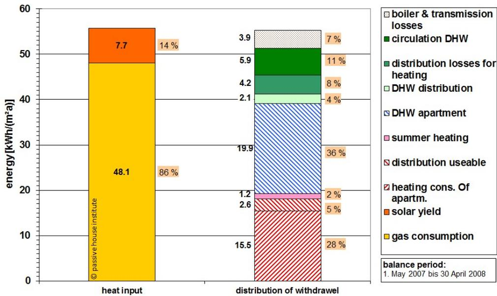
Fig. 9: Energy balance of a Passive House building with 19 apartments with centrally supplied heat from the study by [Peper/Grove-Smith/Feist 2009]. The heat supply and heat applications could be broken down in detail in metrological terms. Interestingly, the annual total for this object is of the same scale as that of the Passive House building sites of the Bahnstadt district in Heidelberg studied in this article.
