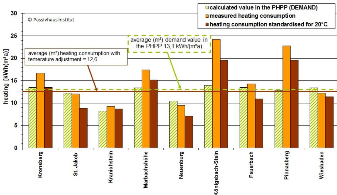
**Fig. 13: Measured heat consumption in comparison with the projected value of terrace, semi-detached and multiple-family houses built to the Passive House Standard. The value determined in the PHPP was calculated for an indoor temperature of 20°C (from [Peper 2008])**
