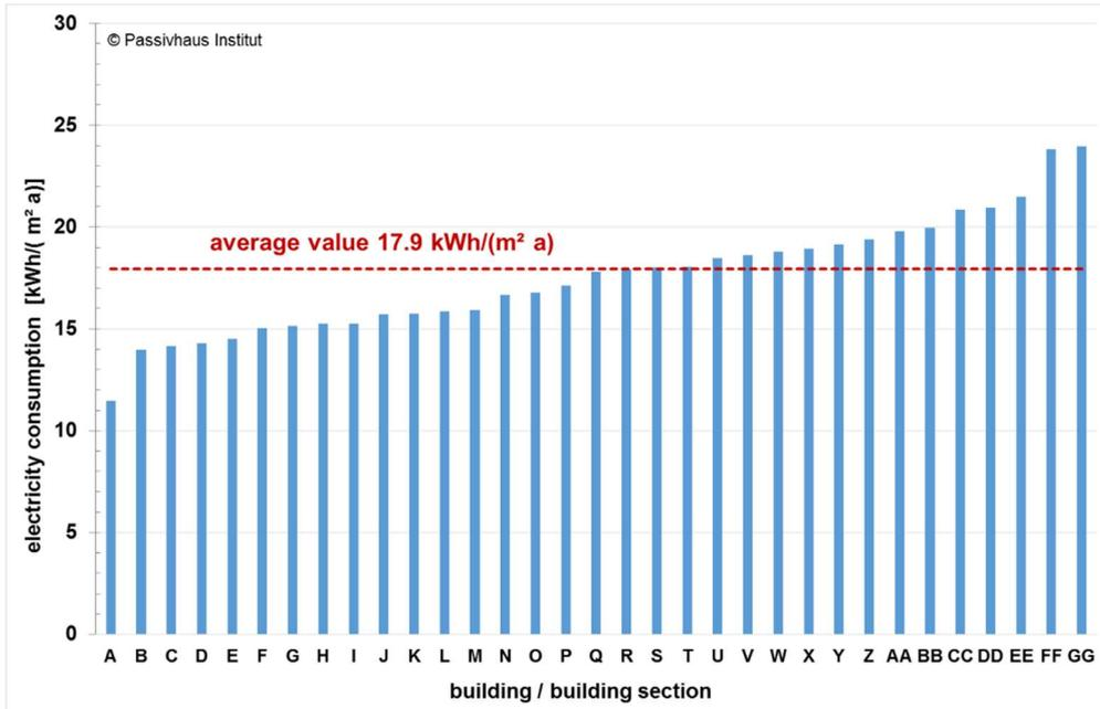
**Fig. 21:** Specific electricity consumption of the 33 buildings or building sections (house entrances) in the Bahnstadt district of Heidelberg with primarily residential use in the year 2015, sorted in ascending order. The consumptions of the apartment meters are shown WITHOUT the common electricity. (The electricity for the ventilation systems is included only for the small number of terraced houses). The area-weighted average value is 17.9 kWh/(m²a).
