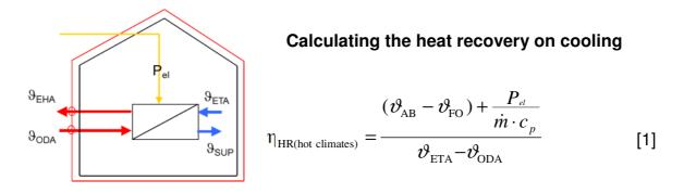
b) Alternatively, the measurement can also be performed under outdoor air conditions
